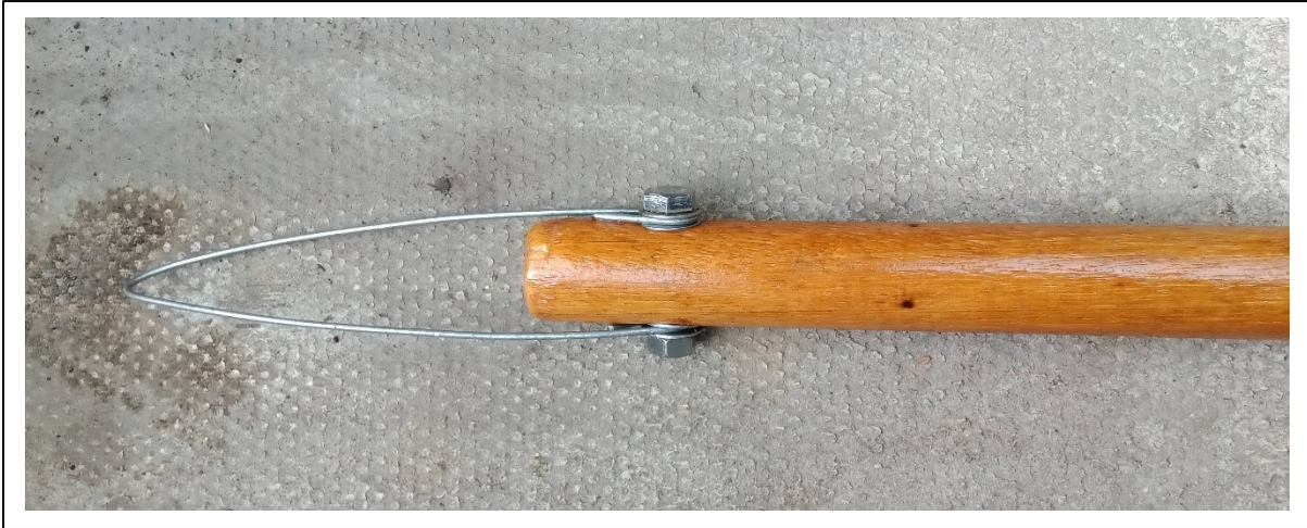
Figure 2. De-hooker or disgorging for removal of circle hooks in reverse in the water, pole length sized to suit boat freeboard
