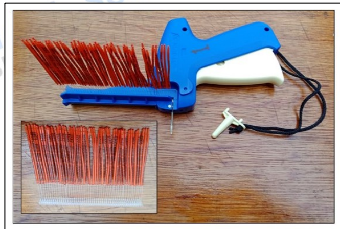
Figure 8. T-Bar tagging gun, loaded and ready for use Inset: Strip of T-Bar Anchor tags for loading
